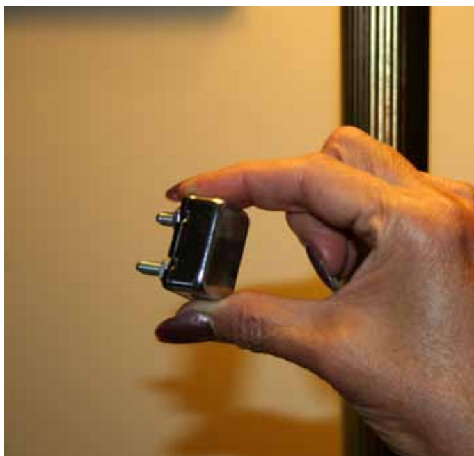
The solution to our stalling problem. A very small circuit breaker.
