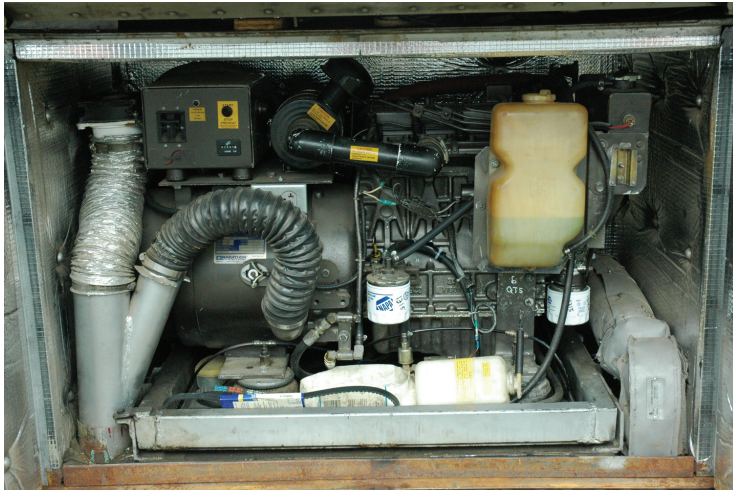
Generator housed in a steel box keeps fire contained while hill climbing outside Salt Lake City
